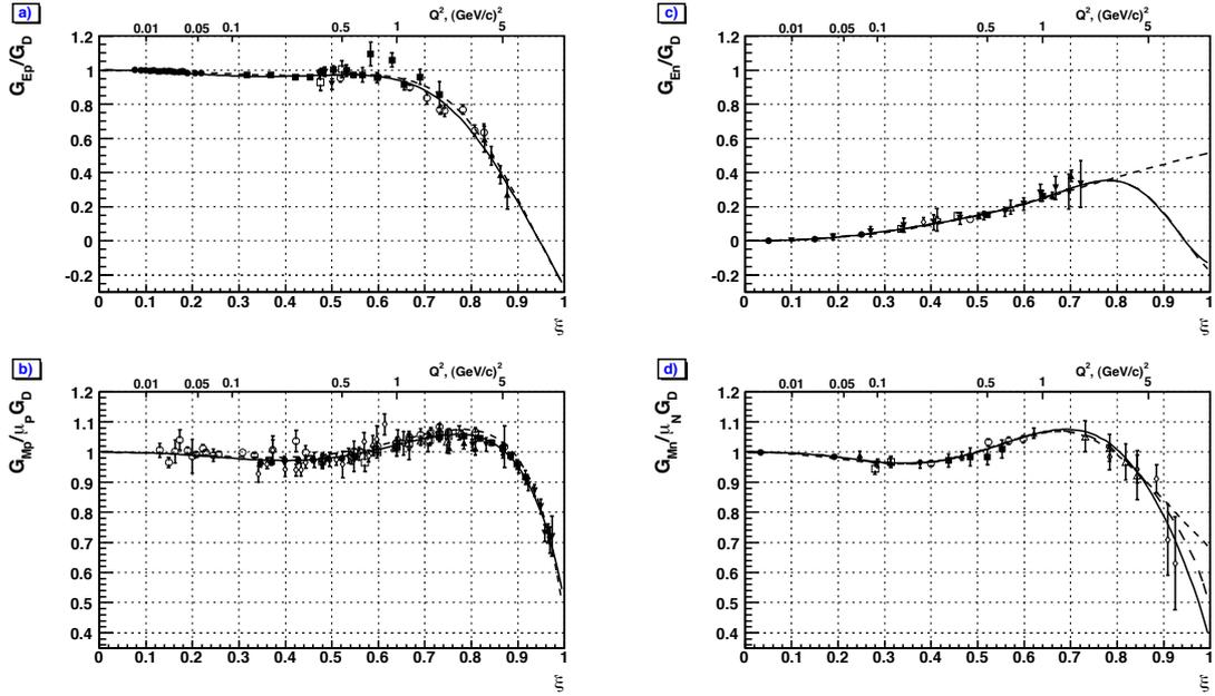
FIG. 1: Ratios of  $G_{Ep}$  (a),  $G_{Mp}/\mu_p$  (b),  $G_{En}$  (c) and  $G_{Mn}/\mu_n$  (d) to  $G_D$ . The short-dashed line in each plot is the old Kelly parameterizations (old Galster for  $G_{En}$ ). The solid line is our new BBBA07 parameterization for  $\frac{d}{u} = 0.0$ , and the long-dashed line is BBBA07 for  $\frac{d}{u} = 0.2$ . The values of  $\xi$  and the corresponding values of  $Q^2$  are shown on the bottom and top axis.
