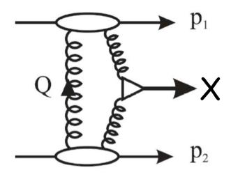
"X" is reconstructed in central detector (ATLAS or CMS) p1 and p2 are tagged by FP420
