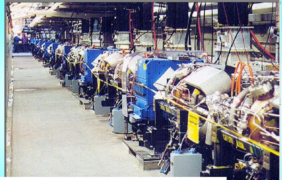
PEP-II: Magnets and RF system are re-usable for SuperB and will be provided by SLAC (negotiations in progress)
