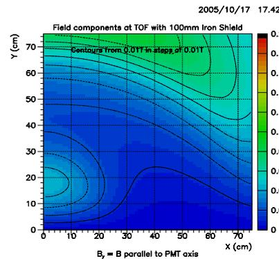
Figure 4:  $B_{//}$  at the position of TOF2 with the 100mm iron shield.
