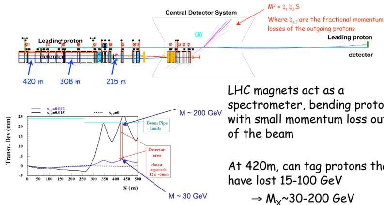
LHC magnets act as a spectrometer, bending protons with small momentum loss out of the beam
