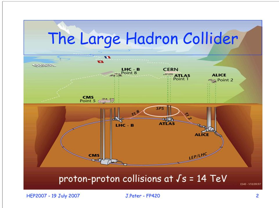
Most of you know what the Large Hadron collider is I expect, but here's a picture of it anyway. It's a proton-proton collider being constructed underground at CERN near Geneva, Switzerland. The proton beams will be accelerated to 7 TeV each for a centre-of-mass energy of 14 TeV, which we expect, or at least hope, to be enough to create any new particles that might be lurking out there.
