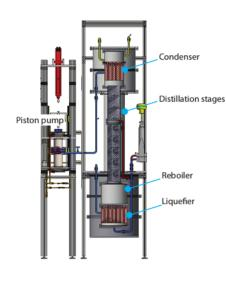
RADON DISTILLATION COLUMN
