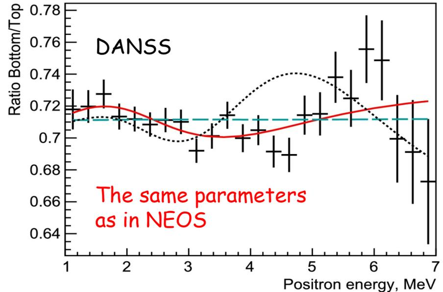
Ratio of positron energy spectra measured at the bottom and top detector positions (stat. errors only). Dashed curve - the three active neutrino case, the red solid curve - the best fit in (3+1) case, the black dotted curve is the RAA expectation.
