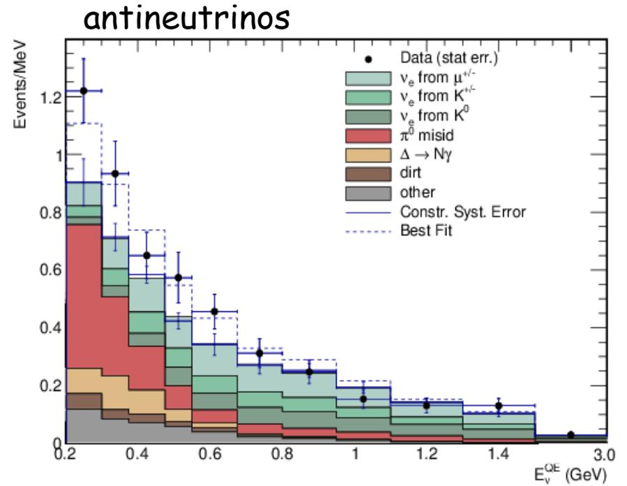
The antineutrino mode  $EQEv$  distributions, with  $11.27 \times 10^{20}$  POT data,  $\nu_e$  CCQE data (points with statistical errors) and background (histogram with systematic errors).
