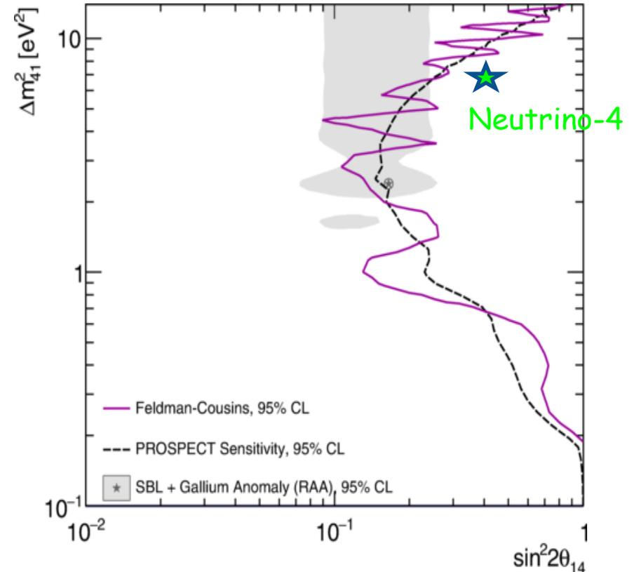
PROSPECT sensitivity and neutrino oscillation exclusion contour with 33 live-days of reactor-ON data Ashenfelter et al.
