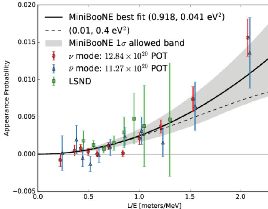
A comparison between the  $L/EQEv$  distributions for the MiniBooNE data excesses in neutrino mode .
