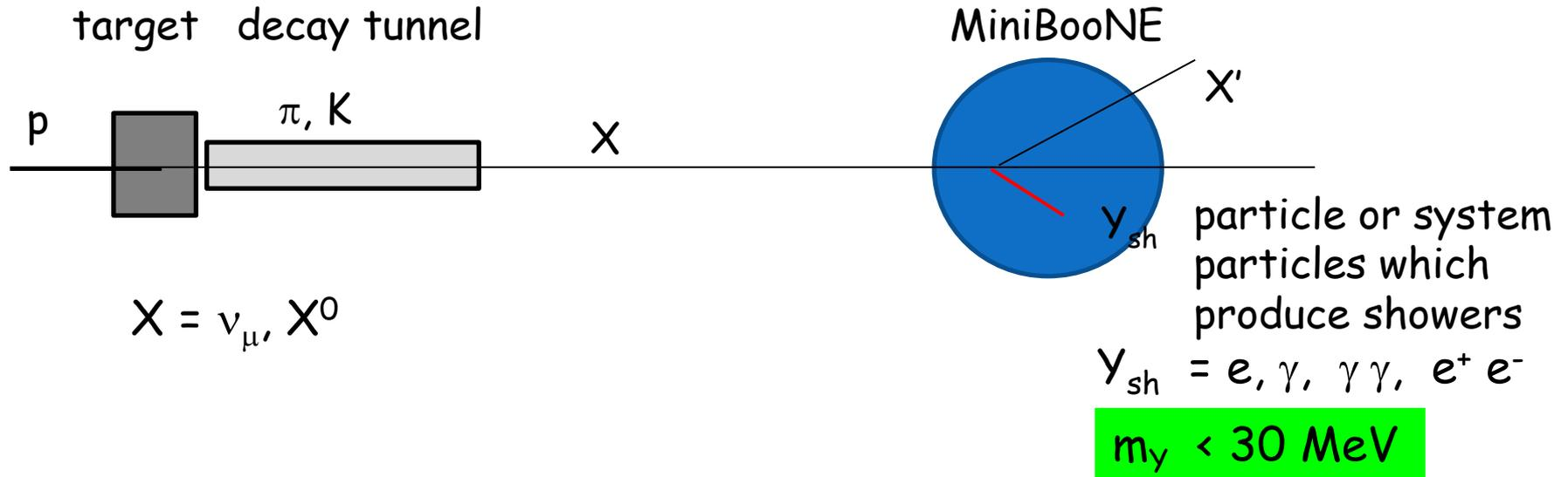
$X^0$  from proton interactions in target restricted by the beam-dump mode (search for DM)
