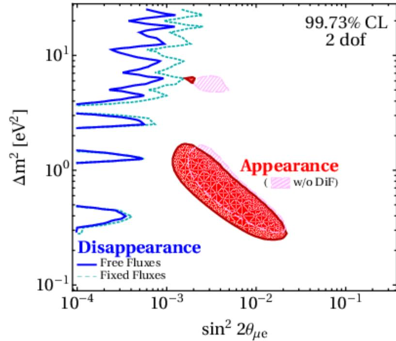
99% CL exclusion curves from various experiments vs. the allowed regions inferred from combination of  $\nu_e$  (bar) disappearance and  $\nu_\mu \rightarrow \nu_e$  appearance data with free (red) and fixed Huber-Mueller (pink) reactor fluxes.
