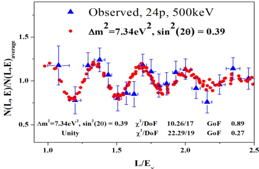
L/E dependence for Neutrino-4 data points vs. expected oscillation signal for the best fit values (red dots), Serebrov 2019.
