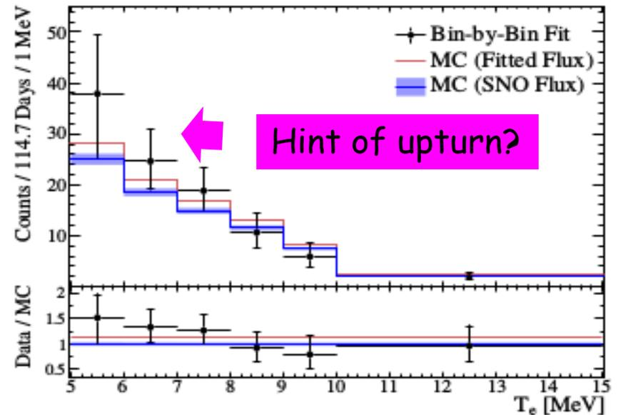
The extracted event rate as function of reconstructed electron kinetic energy
