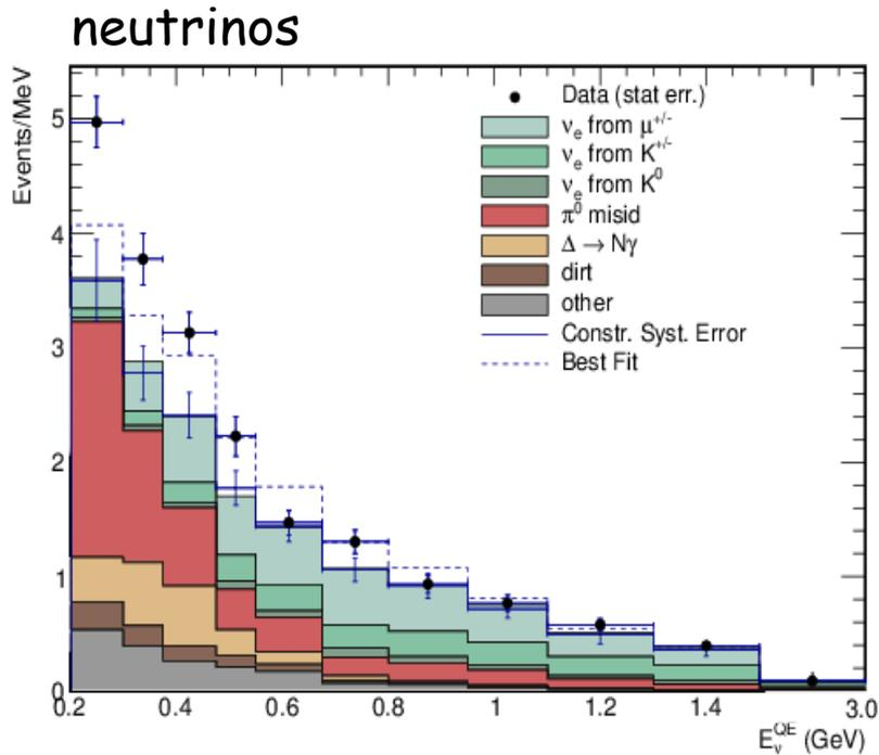
The neutrino mode  $EQEv$  distributions, with  $12.84 \times 10^{20}$  POT data,  $\nu_e$  CCQE data (points with statistical errors) and background (histogram with systematic errors). The dashed curve shows the best fit to the neutrino mode. The last bin is for the energy interval from 1500-3000 MeV.
