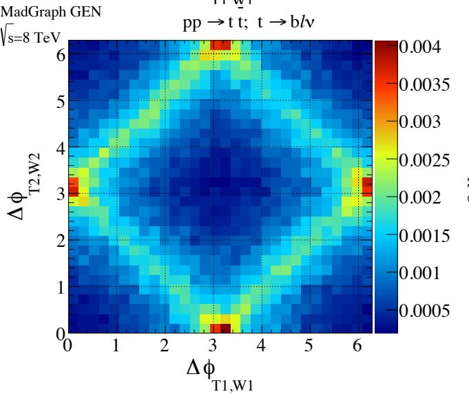
The azimuthal angle between the the top and W decay planes from each hemisphere
