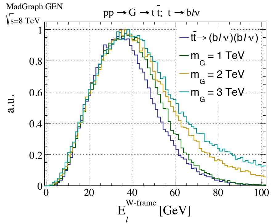
distributions of top/W/neutrino mass-splitting-sensitive observables are nearly identical since graviton signal and non-resonant background both contain on-shell tops
