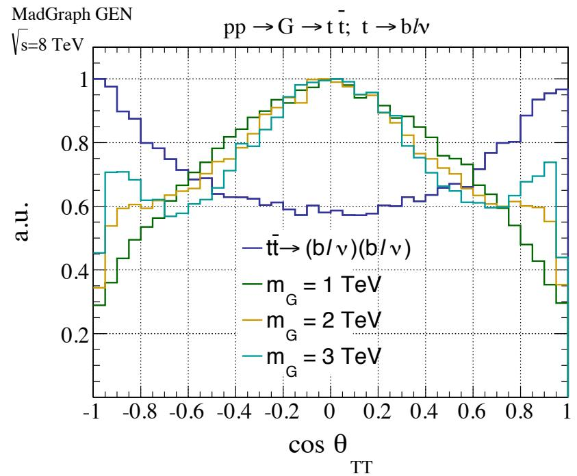
Instead, observables related to the production of the two tops are sensitive to the intermediate resonance
